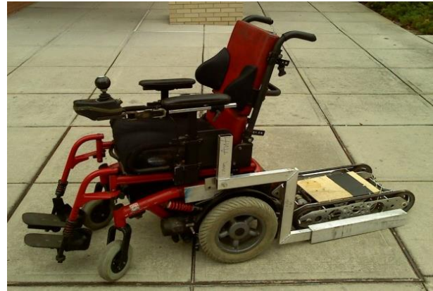
Fig. 18.1. The Deployable Base Attached to a Wheelchair.
