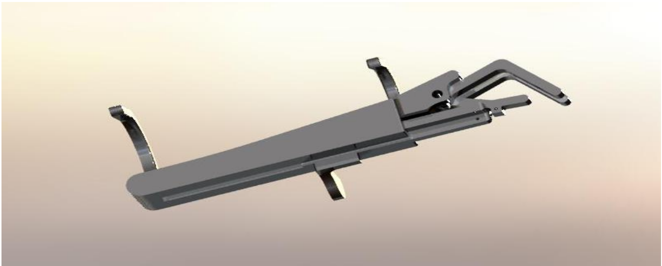
Fig. 18. 31. Part of the Prototype that Allows the User to Take to Cup to the Mouth.
